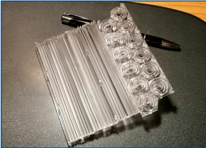
LED - Lens (CNC-milled & polished)
