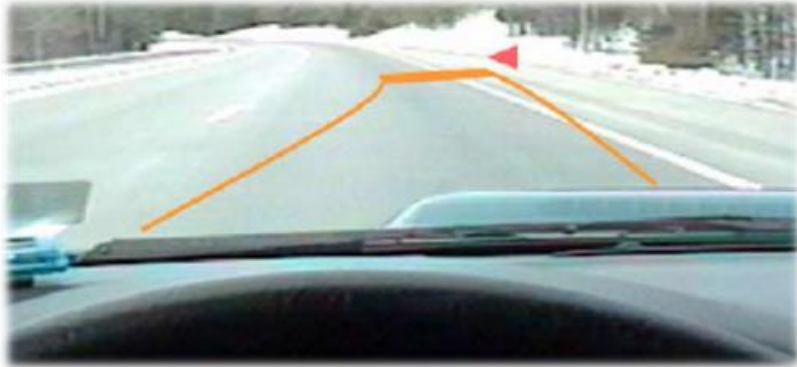
Braking distance indicators for forward collision warning and lane markings for lane departure warning
